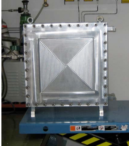
Fig. 20: The finished DENEX-300TN/B detector
